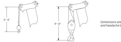
Dimensions are for largest Grove furnished hookblock and headache ball, with anti-two block activated.
