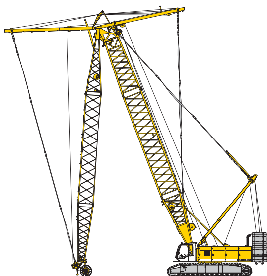
Erecting of main boom and luffing jib
