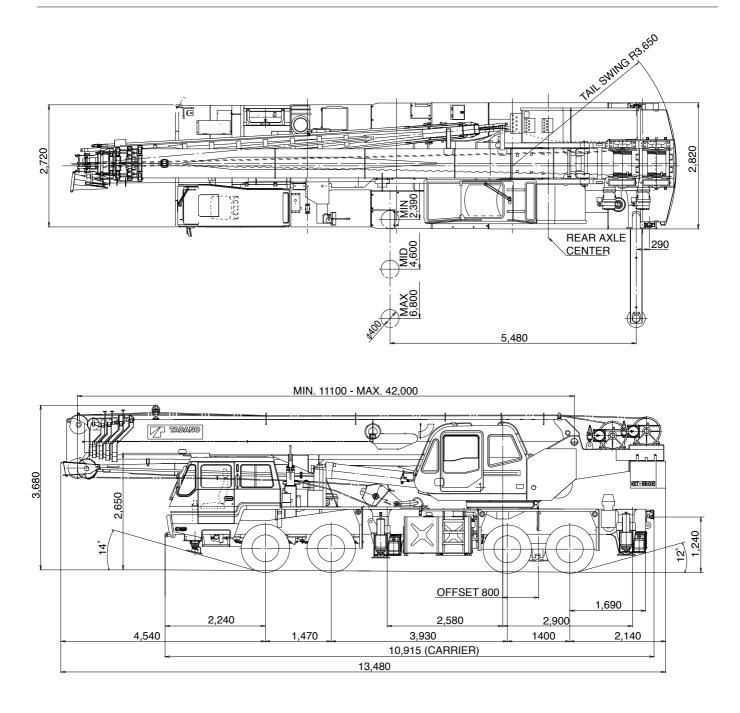
Tread (track) - Front ...... 2,250 mm - Rear ...... 2,110 mm Min. ground clearance ...... 230 mm (rear equalizer beam)
