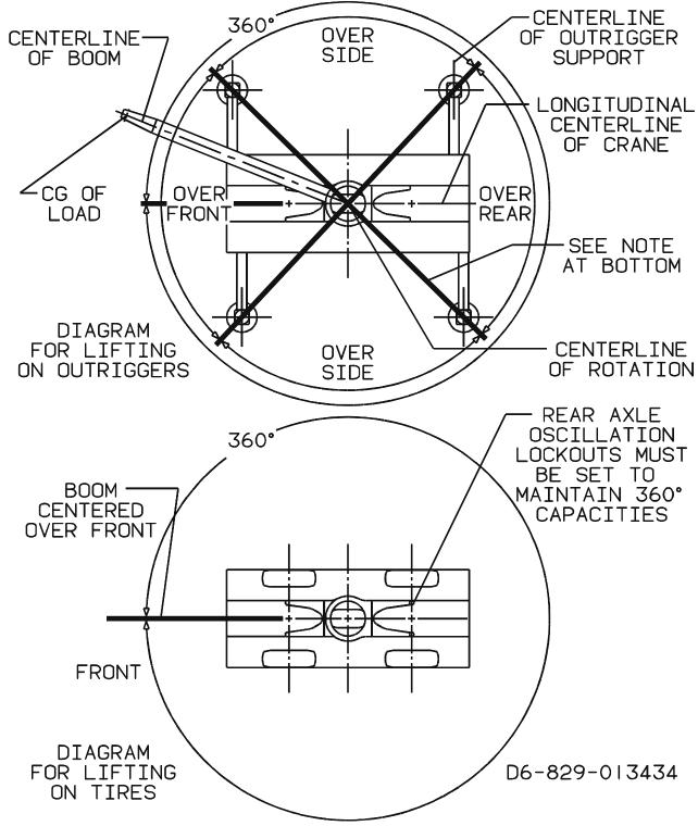
BOLD LINES DETERMINE THE LIMITING POSITION OF ANY LOAD FOR OPERATION WITHIN WORKING AREAS INDICATED WORKING AREA DIAGRAM
